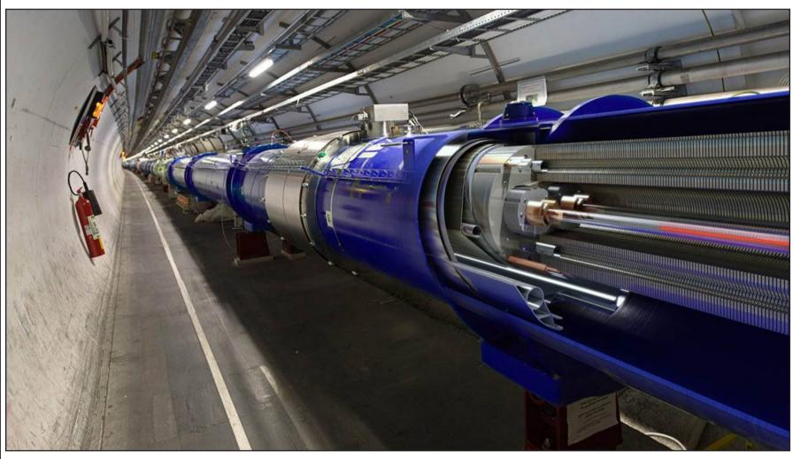
**New Dehli:** A 3D cut-out of the Large Haldron Collider's magnetic dipole. (Image credit: CERN)
